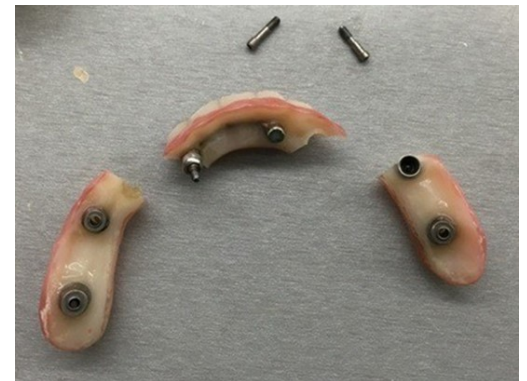
Figure 21: Note the fracture locations where the framework was too narrow and weak. Image from Bauersmiles.com
