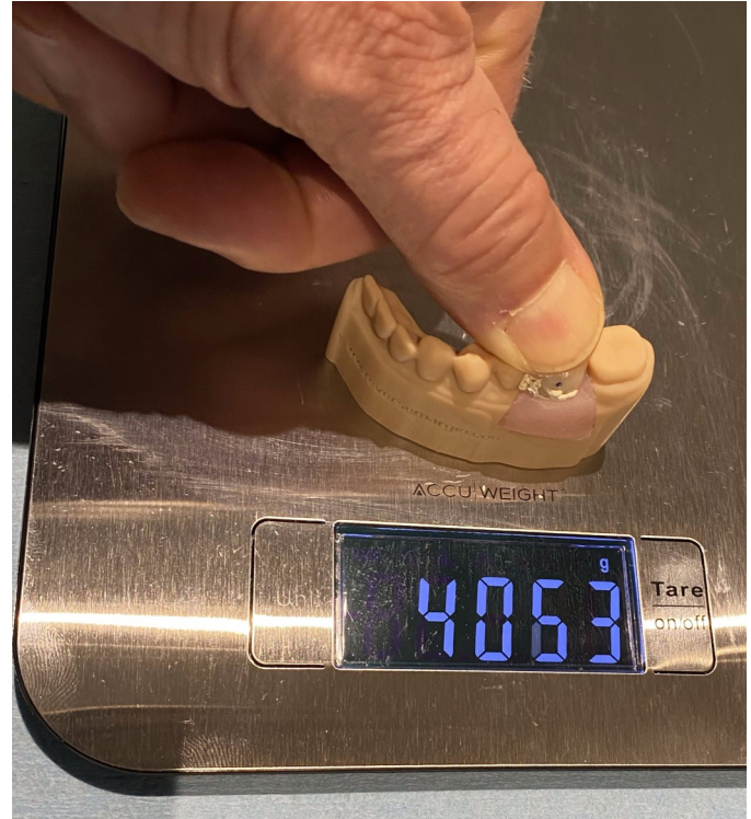
Figure 6: Crown being cemented onto abutment while on a weigh scale. The scale reads 4.053 Kgs.
